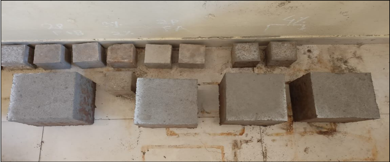
Fig. 5: (a) Casting of One-Part Geopolymer Cubes
