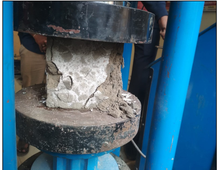
Fig. 7: (c) Testing of Geopolymer Concrete Cube under CTM
