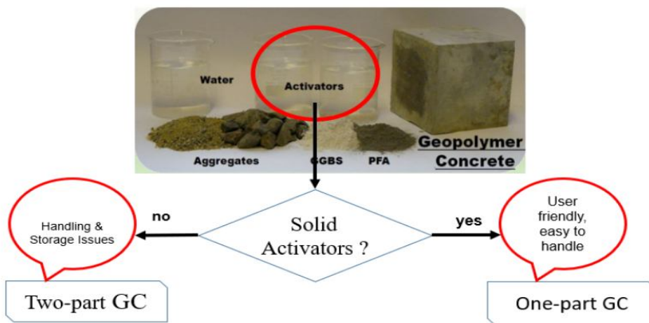
Fig. 3: Two-part & One-part Geopolymer Concrete
