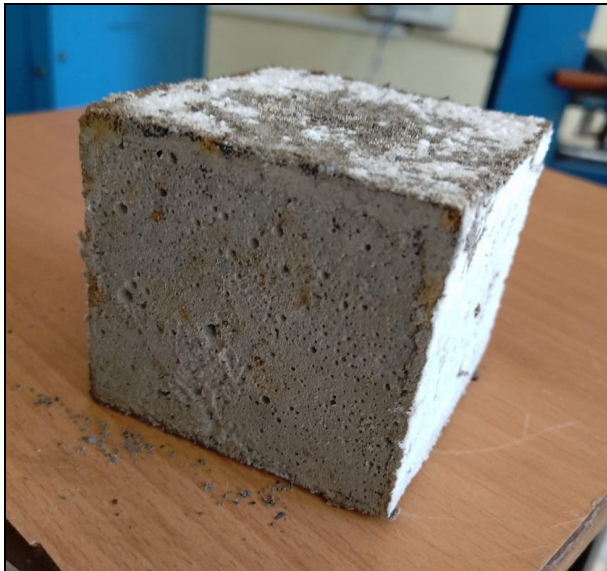
Fig. 6: (b) Demolding of Geopolymer Concrete Cube
