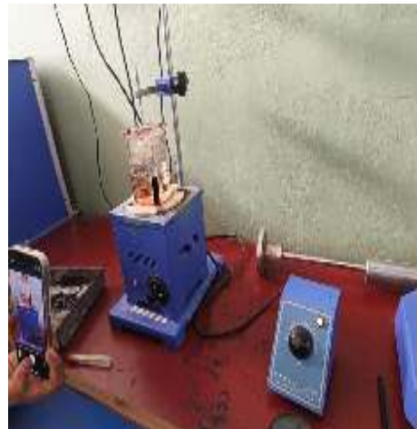
Fig 2 Softening Point Test
