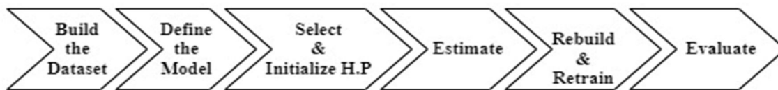
Fig 5: Elementary Framework of Hyper Parameter Optimization (HPO)
