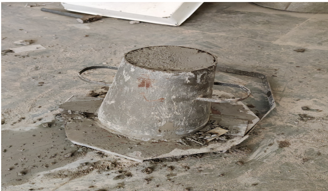
Fig. 6 A Slump cone test
