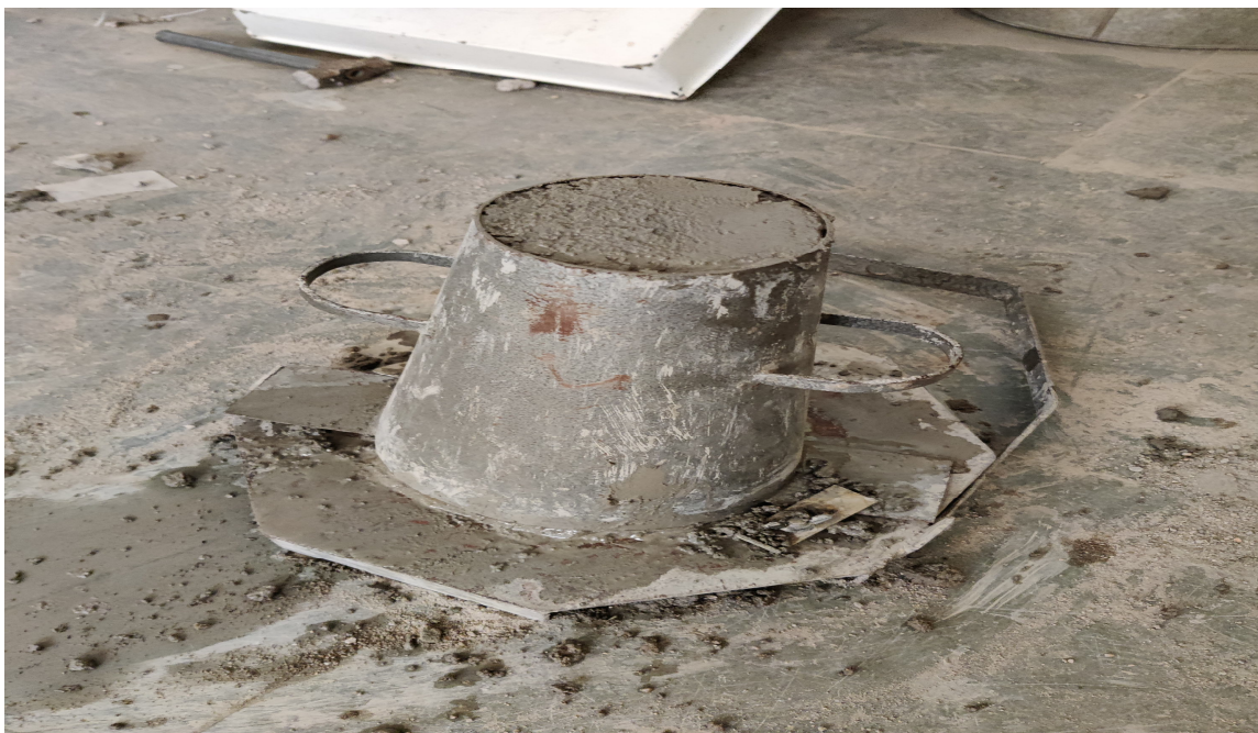
Fig. 6 A Slump cone test
