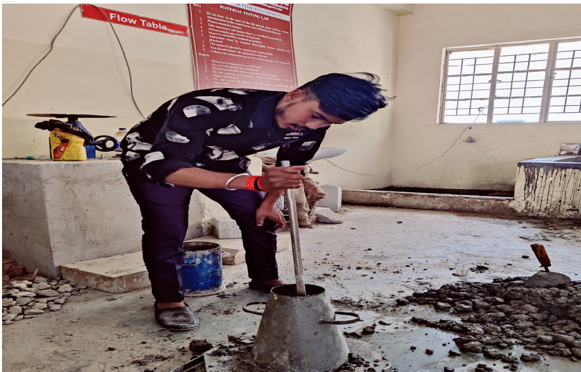
Fig. 5 A Slump cone test
