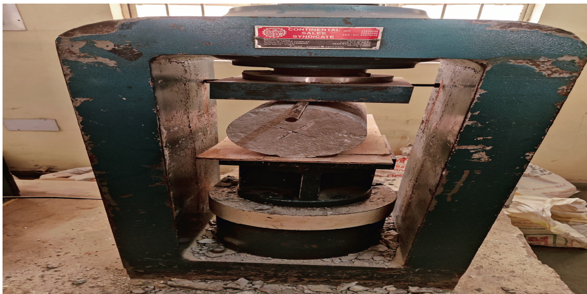
Fig. 2 Compressive strength of cylinder
