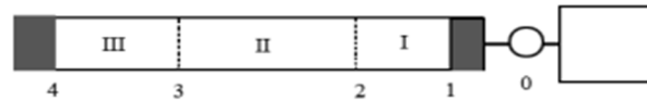
Fig.4 Sections of gas in the pulse tube. The regenerator is on the left side of region III the orifice is at point 0 which leads into a reservoir.
