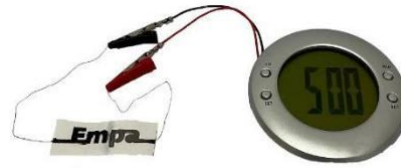
Fig:3. Paper battery by powering the display of an alarm clock.
