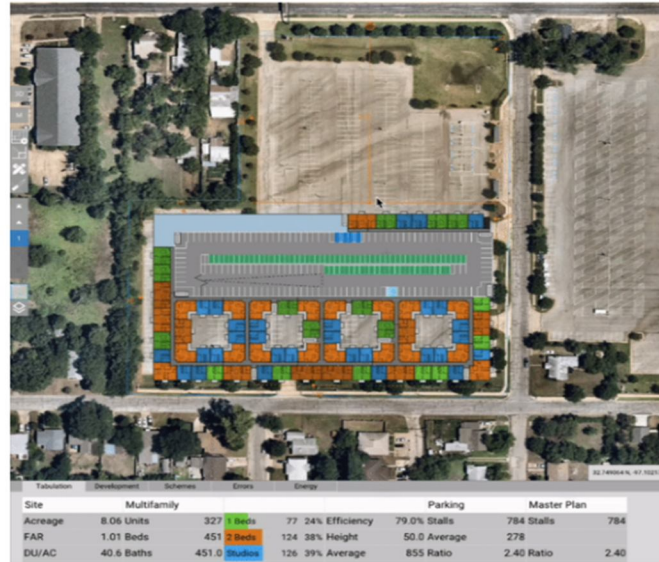
Fig 7 : The 'TestFit' creates the building's massing based on real-site GIS data using algorithms and artificial intelligence (AI) (Tovar, 2023)
