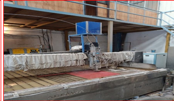
Fig.2 Abrasive water jet machine experimental setup
