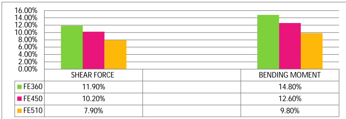
Fig. 4.5 : Effect of grade of steel in Z-section
