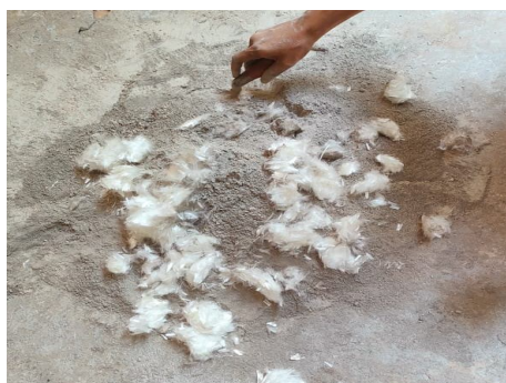
Fig. 1 ECC Mix Preparation
