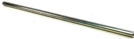
Fig. No. 4.5 Tamping Bar
