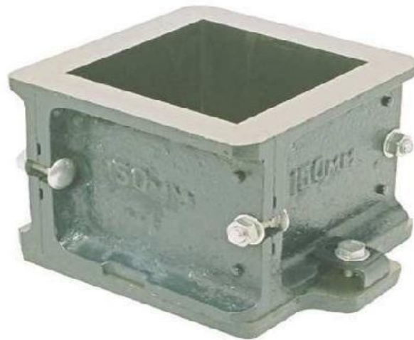
Fig. No. 4.2 Cube Mould
