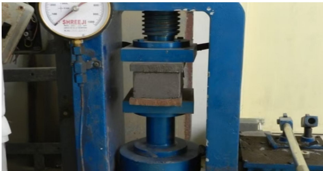
Figure 5. Compressive strength of cube using CTM
