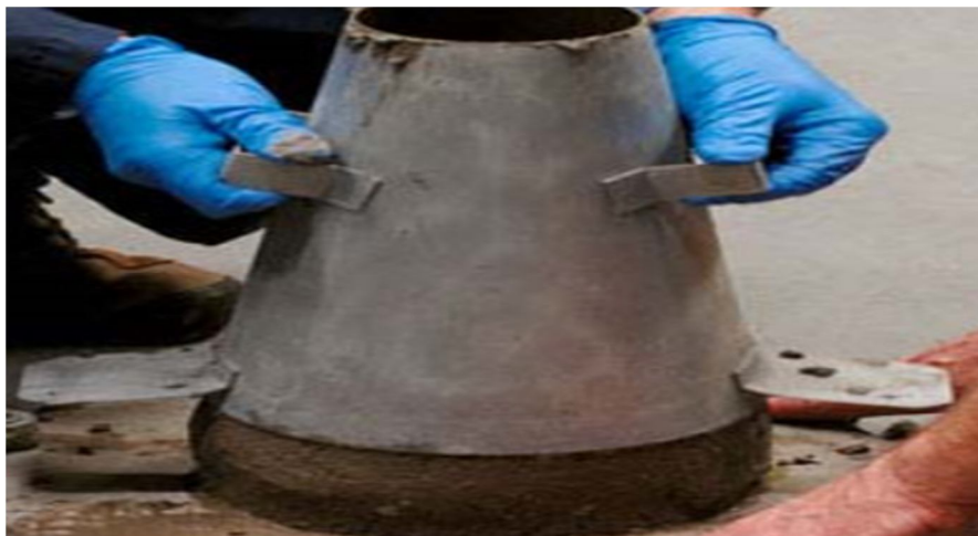
Figure 4. slump cone test
