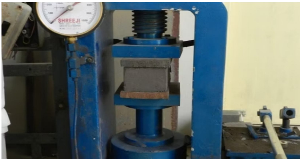
Figure 5. Compressive strength of cube using CTM
