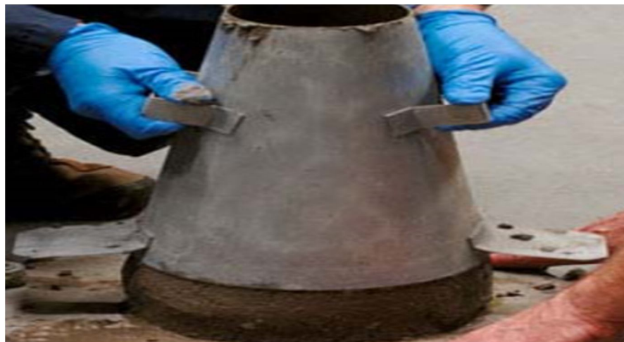
Figure 4. slump cone test
