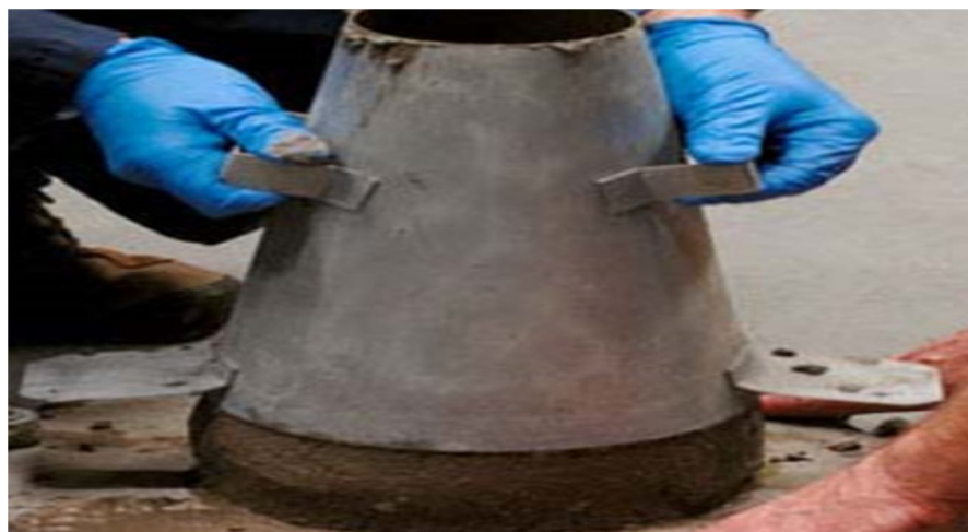
Figure 4. slump cone test
