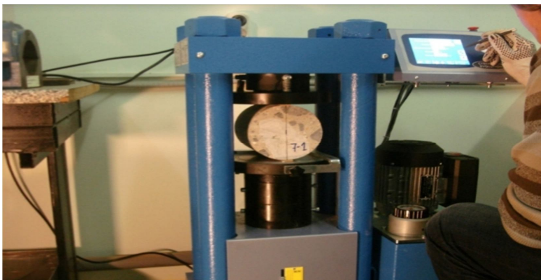
Figure 6. split tensile strength test of cylanders
