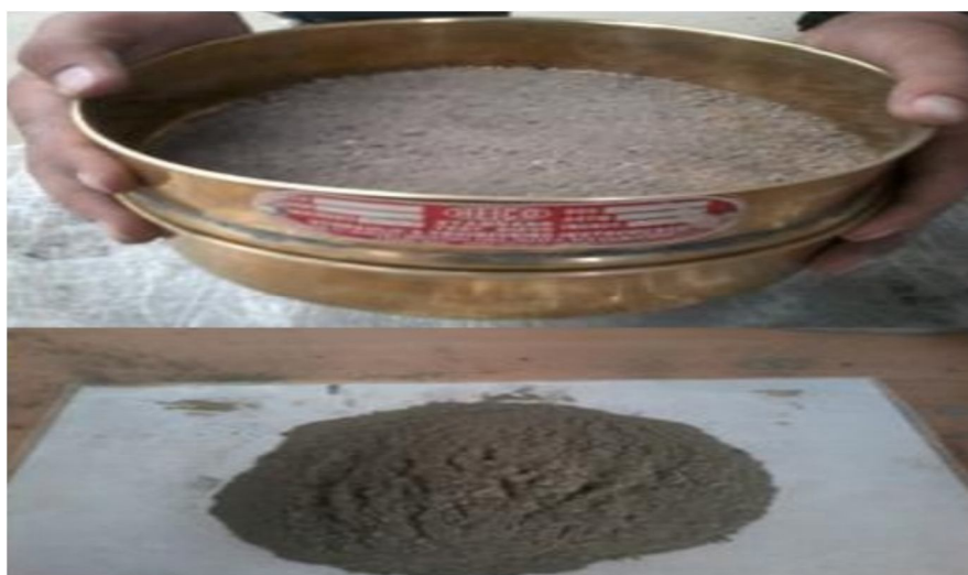
Fig 2: sieving of waste paper sludge ash
