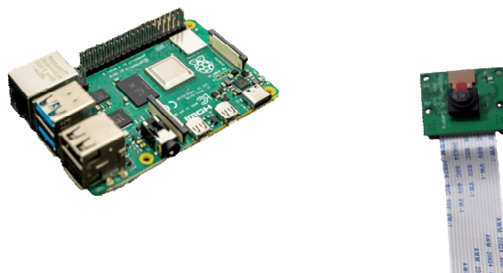
Fig -1: Raspberry Pi 4 and Pi-Cam
