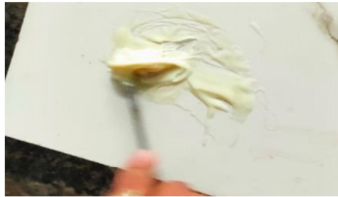
Fig. 8 Mixing of resin with hardener
