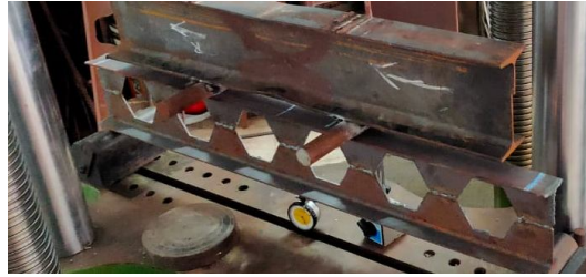
Fig. 12 Test set up of control castellated beam
