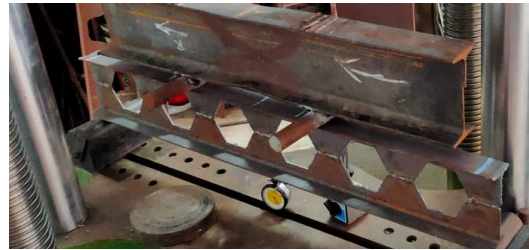
Fig. 12 Test set up of control castellated beam
