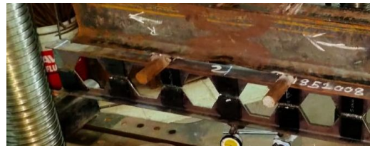
Fig. 13 Test set up of hexagonal castellated beam with transverse CFRP stiffeners
