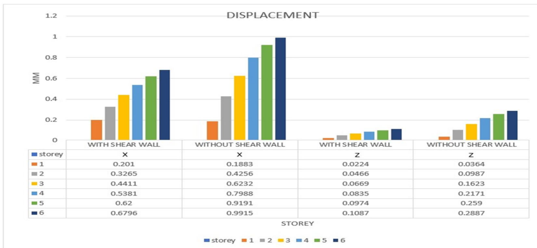
Chart-1: G + 5 Building Displacement in X & Z Direction.
