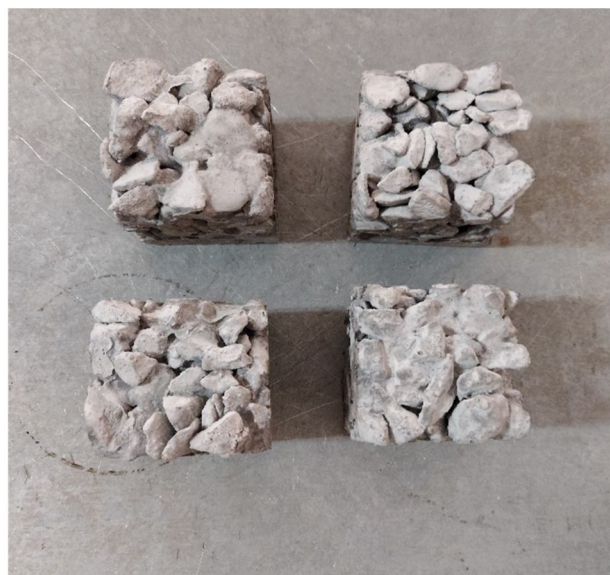
Fig.3.9 Specimen for Cantabro test
