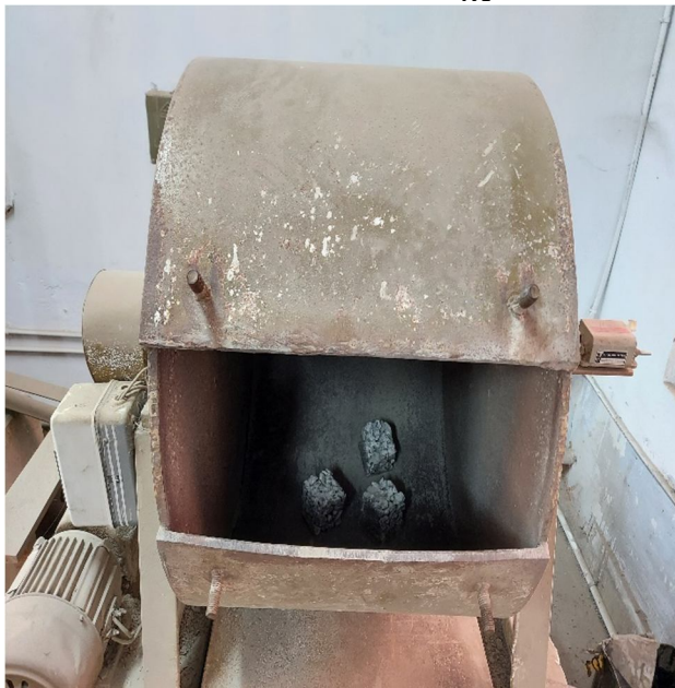
Fig.3.8 Los Angeles Abrasion Machine
