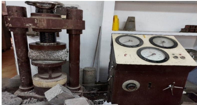
Fig.3.6 Split tensile strength of cylinder
