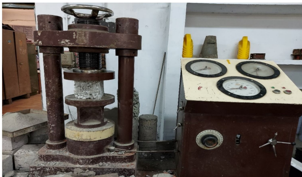
Fig 3.3 Compressive strength on trial mix specimen
