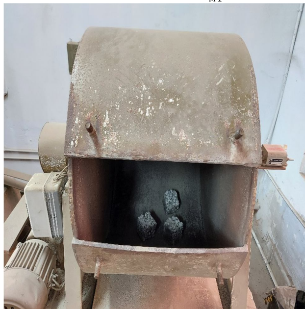
Fig.3.8 Los Angeles Abrasion Machine
