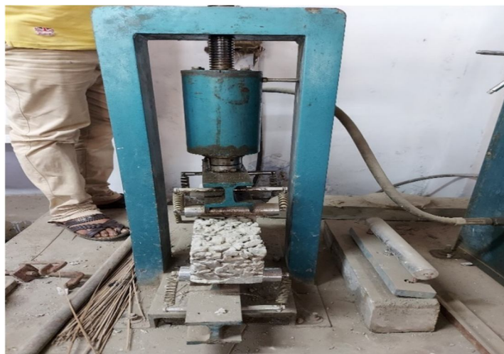
Fig.3.7 Flexural strength test
