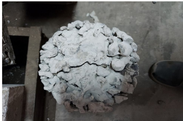
Fig. 4.2 Failure of split tensile strength
