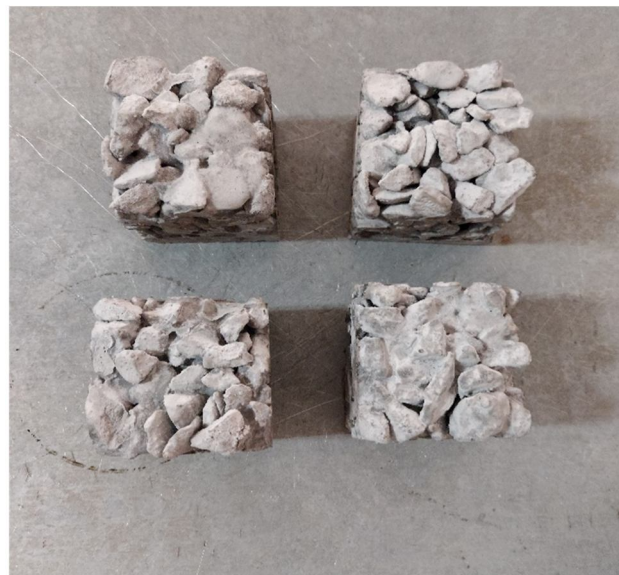
Fig.3.9 Specimen for Cantabro test
