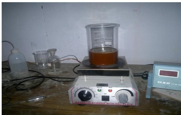
Figure 5 Heating the Lemon Grass Oil After Transesterification Process in Magnetic Stirrer Heater.
