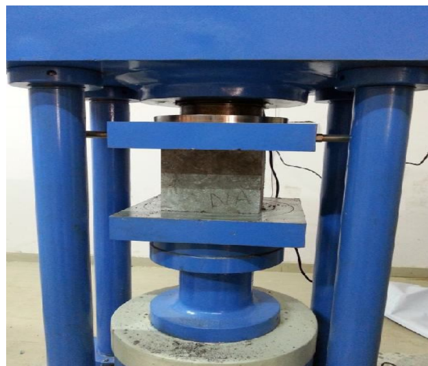
Fig. 7 Compressive Strength Test
