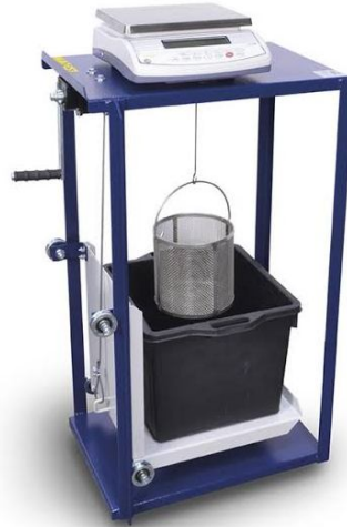
Figure 3.2: Wire mesh apparatus
