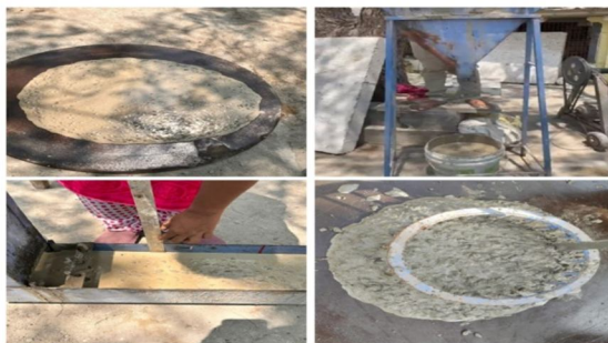
Fig.1 Performing Fresh properties of HVFSCC
