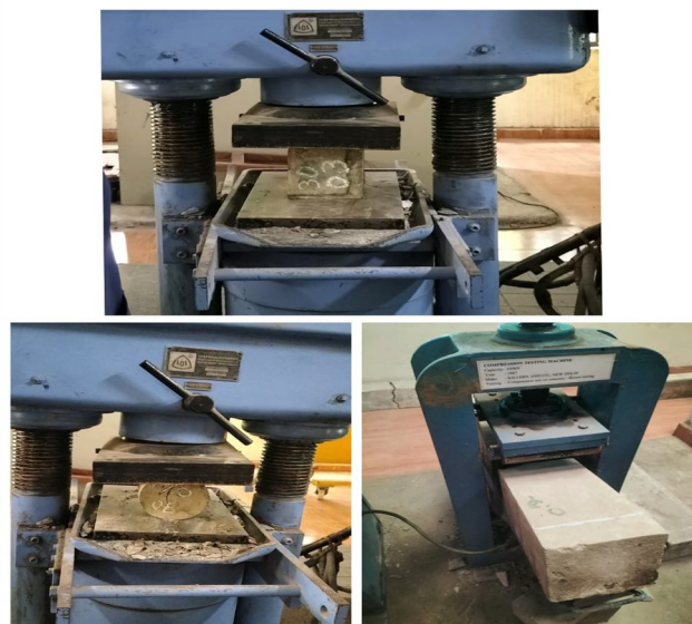
Fig.2 Performing hardened tests on HVFSCC Specimens
