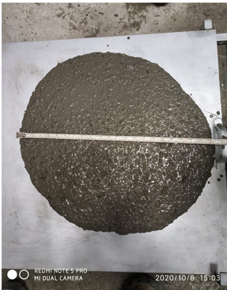
Fig.1 Flow Table Test
