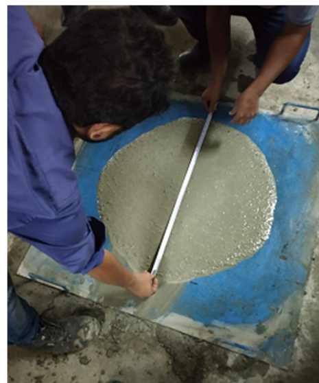
Fig.2 Slump Flow Test
