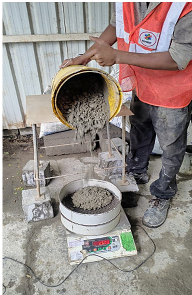
Fig 7. Sieve Segregation resistance Test
