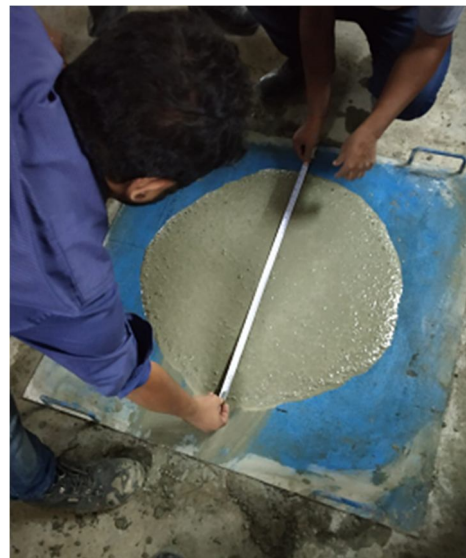
Fig.2 Slump Flow Test
