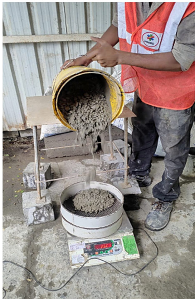
Fig 7. Sieve Segregation resistance Test
