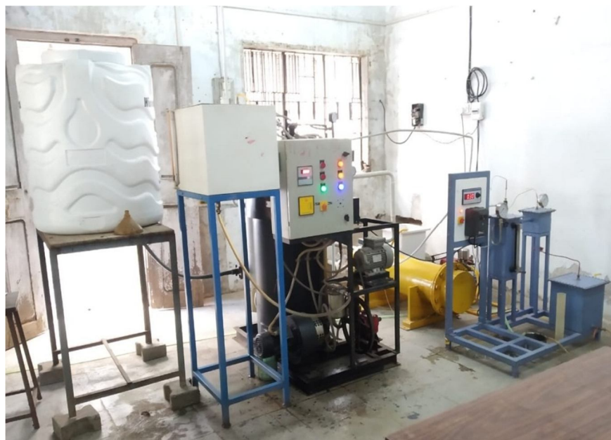
Fig. 1 Boiler setup with condenser and Separating And Throttling Calorimeter
