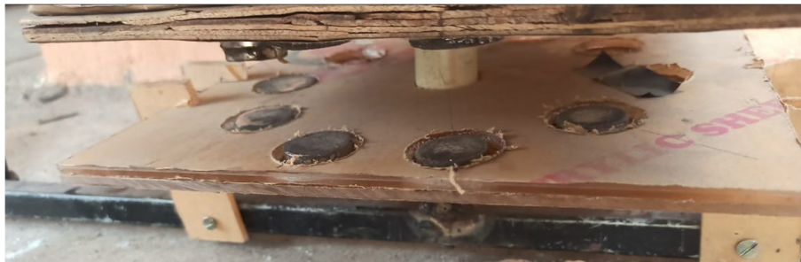
Figure 2 arrangement of both planes holding magnets within 4cm apart
