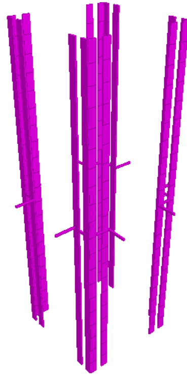
Fig. 13: Shear wall at periphery with 29.05 % opening (Case OSWA5a)
