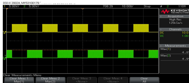
Fig 7: PWM pulse to the SEPIC converter
