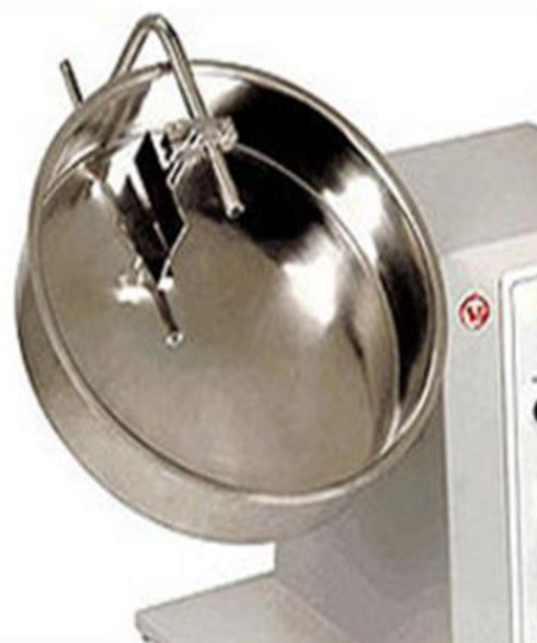
Figure 6. Rotary disk pelletizing equipment
