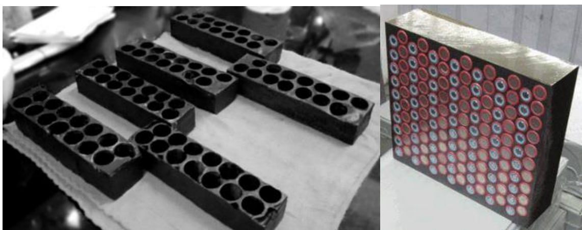
Fig 7. PCM Li-ion Battery Cooling Jackets for passive thermal management of the batteries between 20-40°C [24]
