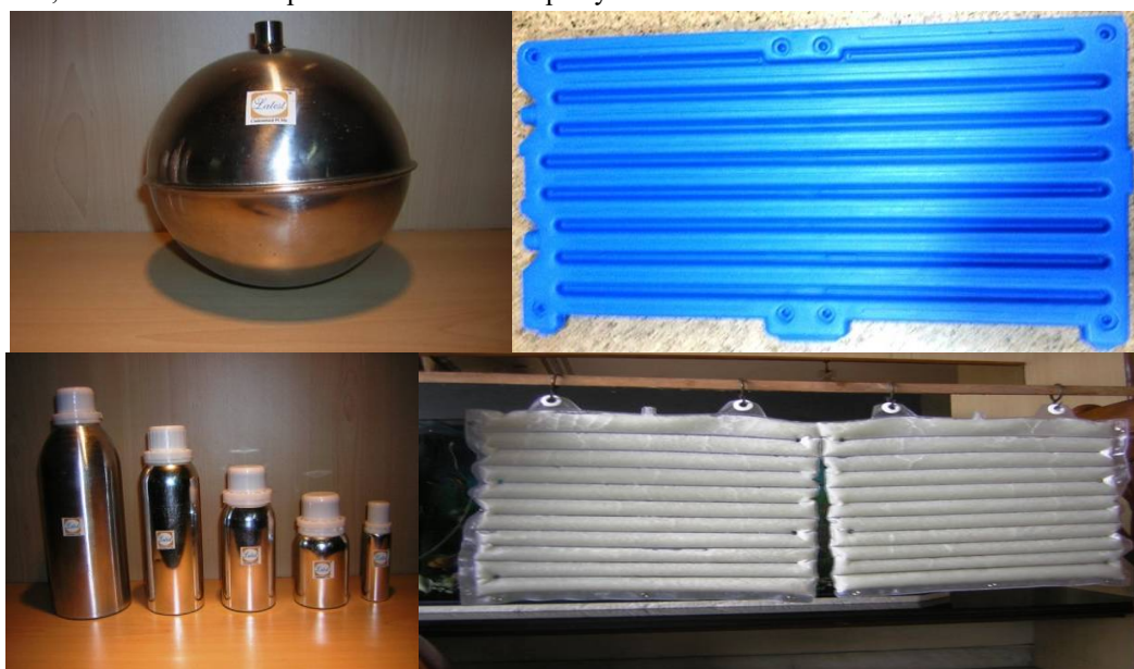
Fig 5. Various methods of PCM containment.
