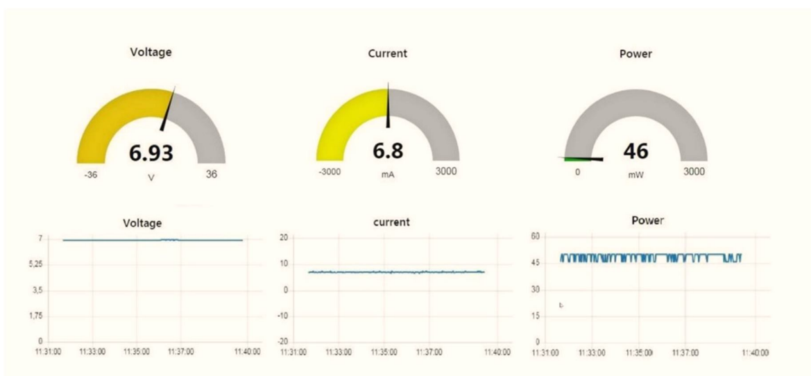
Fig 15: NodeRED dashboard for real-time monitoring
