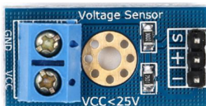
Fig. 5: 25V voltage sensor
