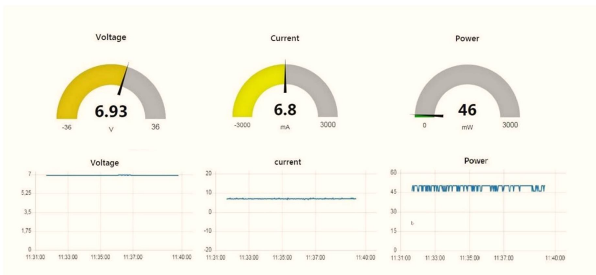
Fig 15: NodeRED dashboard for real-time monitoring
