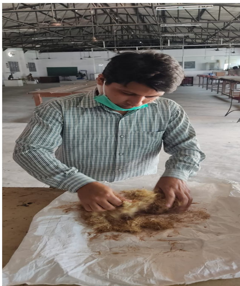
Fig 3.10: Hand Lay Method
