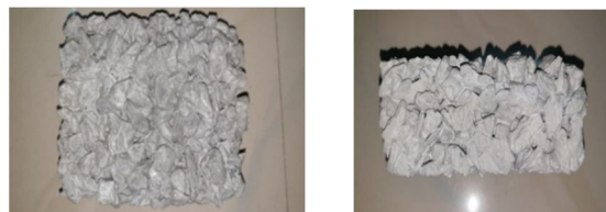
Fig 7 Porous concrete real sample
