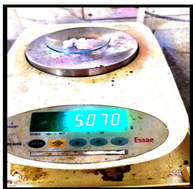
Fig 18: Weighing sodium hydroxide pellets
