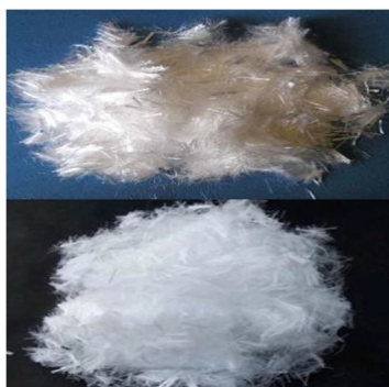
Fig. 3. Various polymer fibers used in concrete
