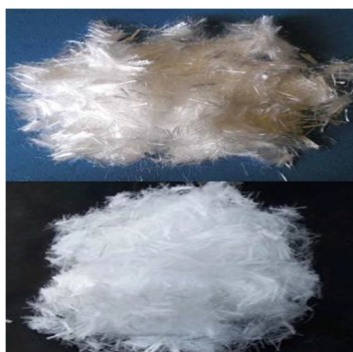
Fig. 3. Various polymer fibers used in concrete
