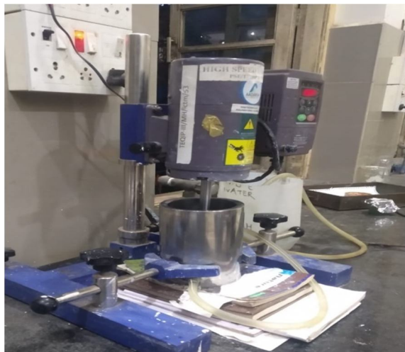
Fig. 2.1 High speed disperser for paint formation
