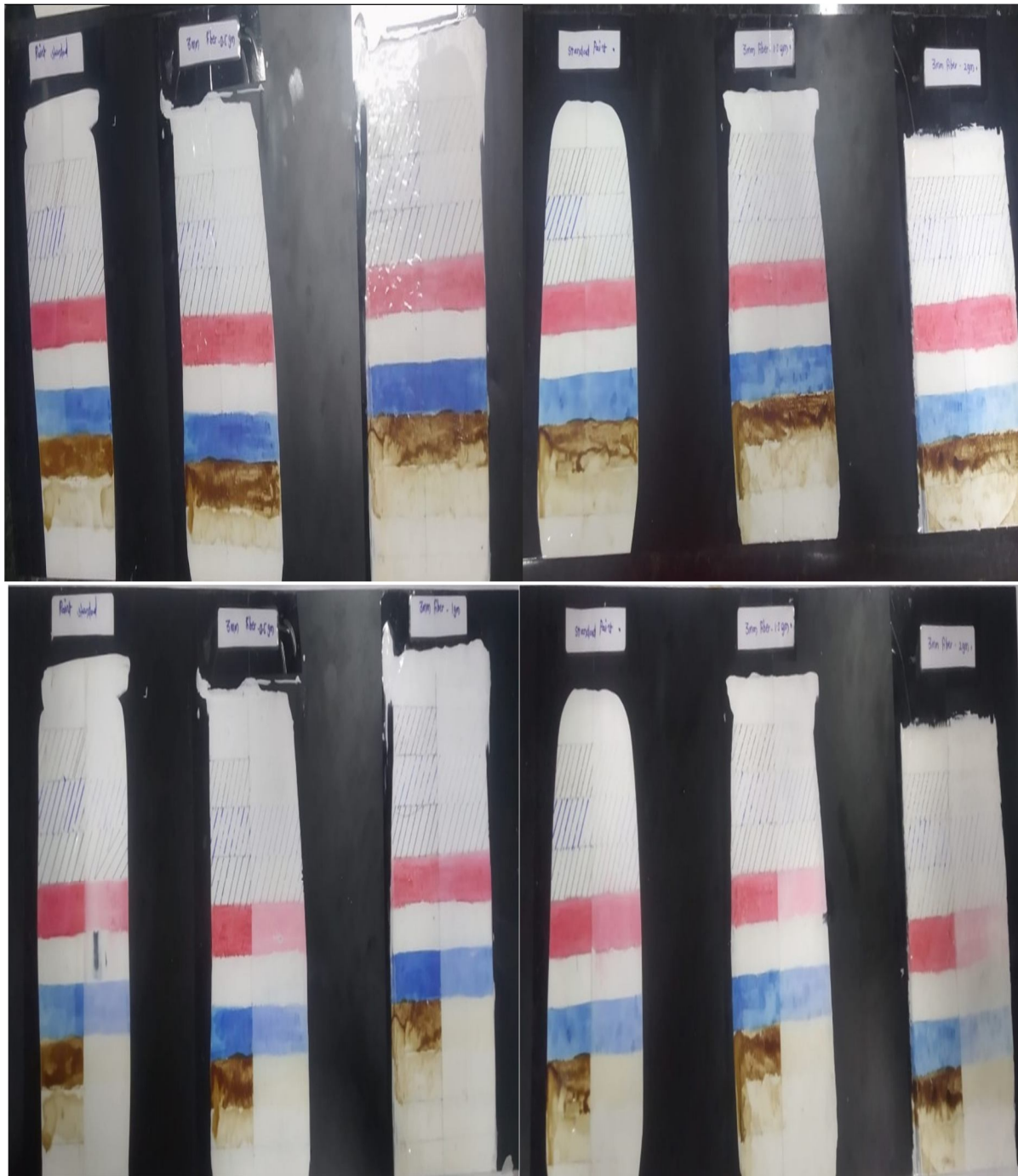
Fig. 5.3 : stain resistance test before and after
