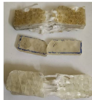
Fig 7: Specimens after Impact Test
