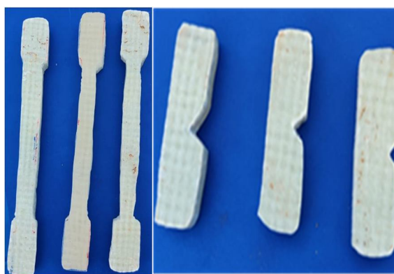
Fig 4: Resin and E-glass fiber Specimens for Tensile and Impact tests
