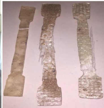
Fig 7: Specimens after Tensile Test
