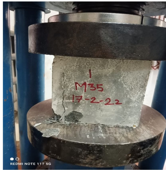
Figure 3. Compressive Strength Test
