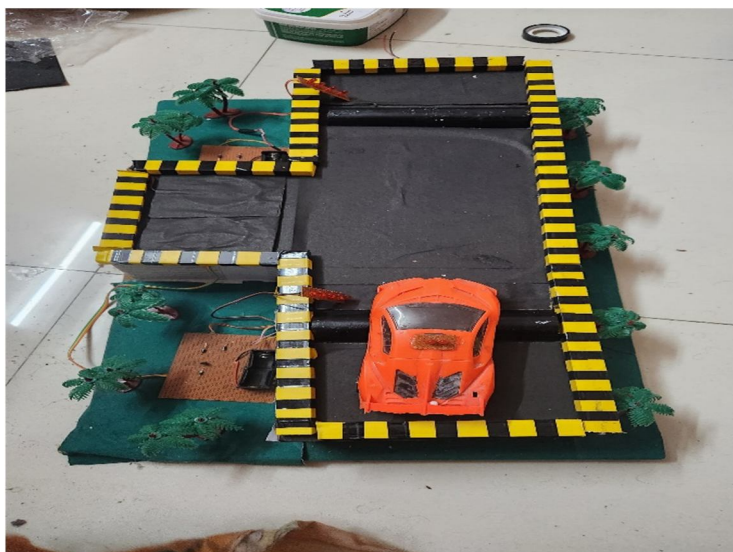
Figure 7 – Car on speed breaker for energy generation
