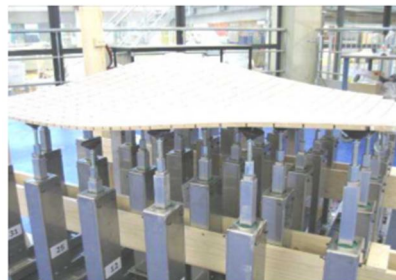
Figure 5. Prototype of a flexible mould built by Rietbergen and vollers
