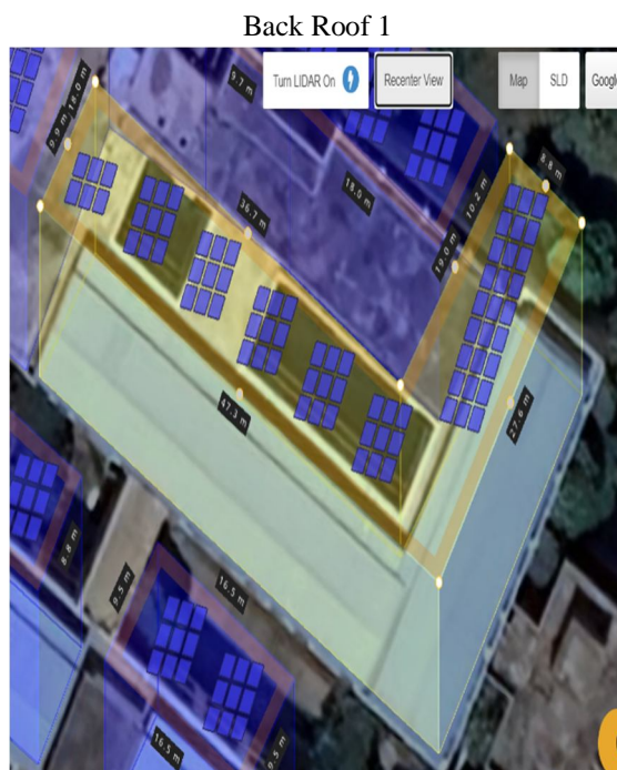
Fig 7 Back Roof 1: 78 modules, 26 KW generation (present in the back side part of the campus building)
