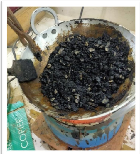
(fig.9:Plastic mix with aggregate and bitumen)
