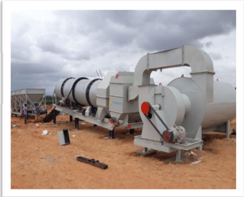
(fig.8:Mixing plant of flexible pavement)
