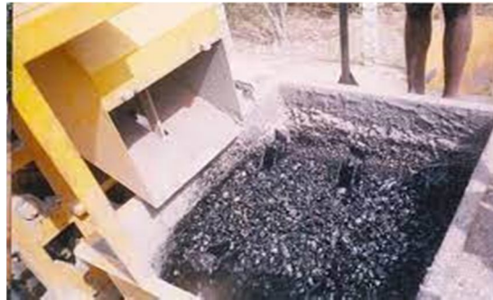
(Fig.3: plastic coated with aggregate and bitumen)
