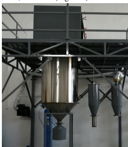
Fig 1. Vertical gas atomization unit designed and manufactured
