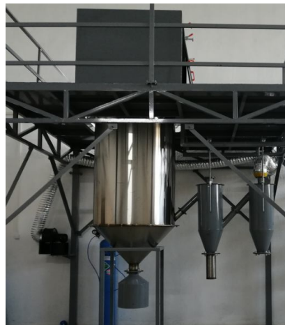
Fig 1. Vertical gas atomization unit designed and manufactured
