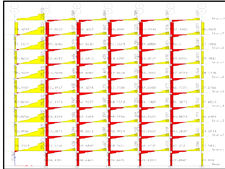
Fig. 5.4: SFD after removal of column C1
