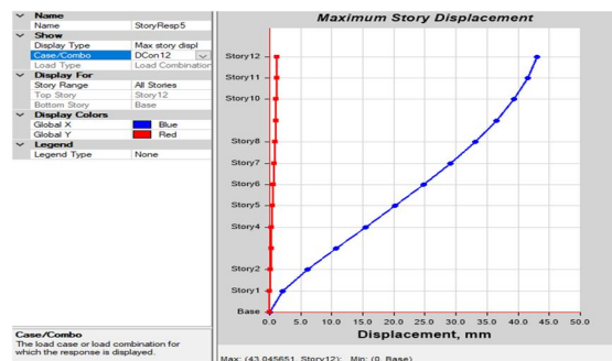
Figure 19 Maximum Storey Displacement Curves For X Direction
