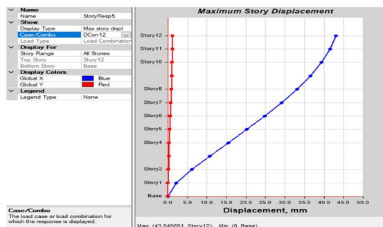
Figure 19 Maximum Storey Displacement Curves For X Direction
