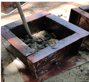
Fig 5. Casting of specimens
