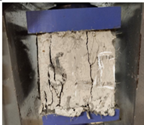
Fig 10. Specimen under compressive test
