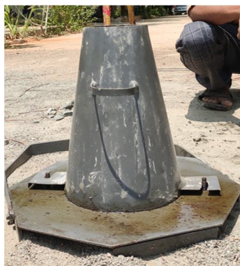
Fig 8. Slump cone test
