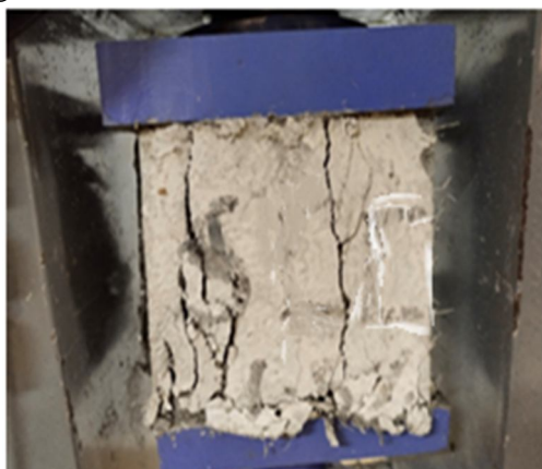
Fig 10. Specimen under compressive test
