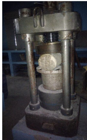
Fig 12. Specimen under Split Tensile Test
