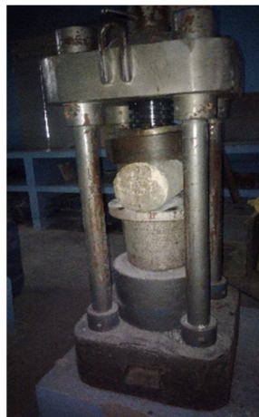
Fig 12. Specimen under Split Tensile Test
