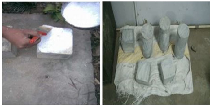
Fig 7. Curing of concrete
