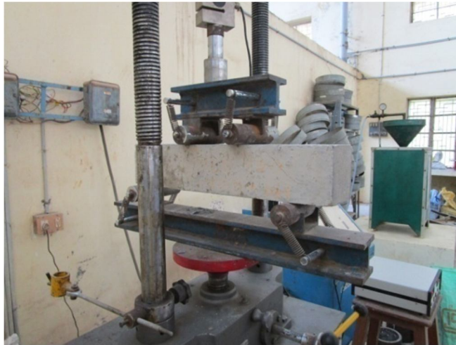
Flexural strength test setup
