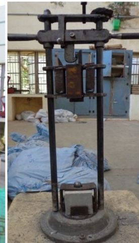
Impact strength test setup
