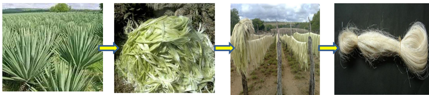
Various stages in processing of the Sisal Fibres
