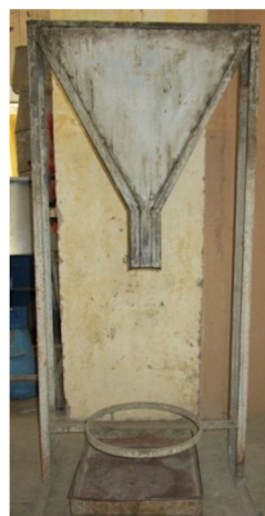
V-Funnel test Setup
