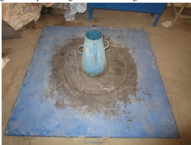
Slump Flow test Setup
