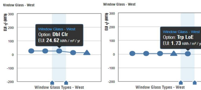
Fig 8: Results are compared of EUI before and after window glazing material alterations
