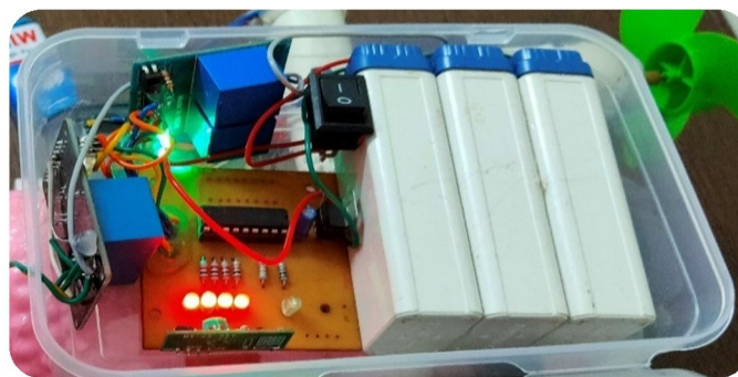
Fig.7 Control unit (control circuit of the submarine which contains battery, receiver unit, etc)
