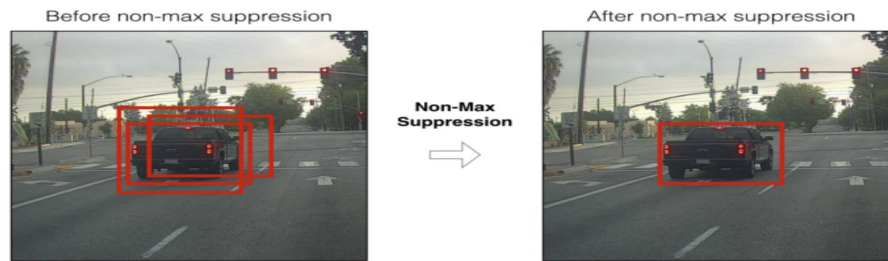
Fig. 2 Before and after Non-Maximum Suppression
