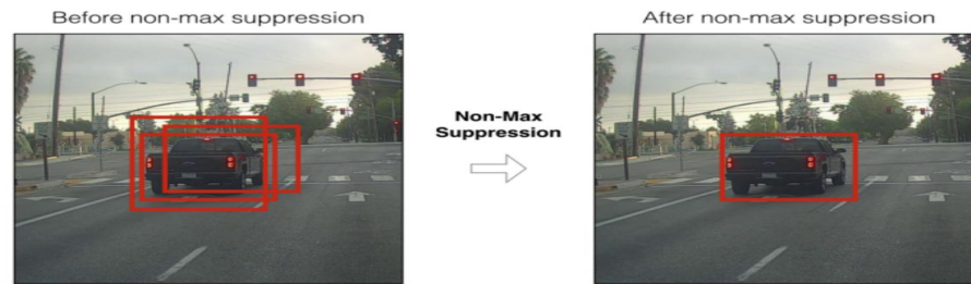
Fig. 2 Before and after Non-Maximum Suppression
