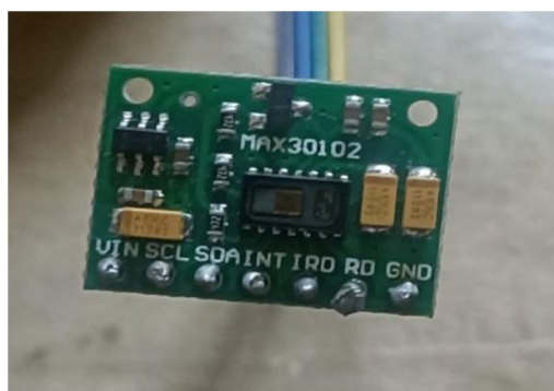
Fig. 4 Pulse Oximeter Sensor
