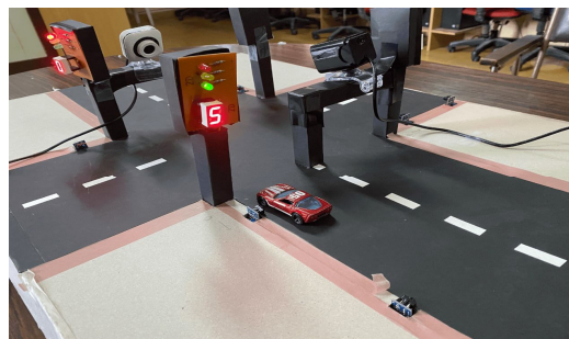
Fig. 5. Traffic lane demonstrating a single sensor trigger
