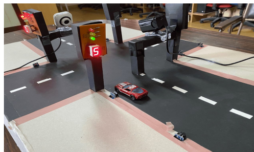
Fig. 5. Traffic lane demonstrating a single sensor trigger
