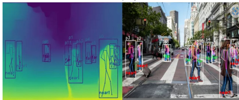
Fig. 5 Classification of the detected pedestrians as "near" or "far"
