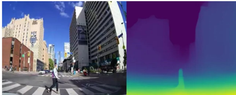
Fig. 3 The depth map of the image produced after MiDaS pipeline.
